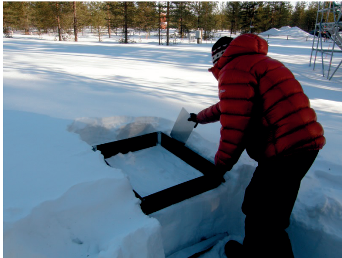
Figure 1. Snow sample was taken from snowpack with a metal bottom plate and a plastic frame
