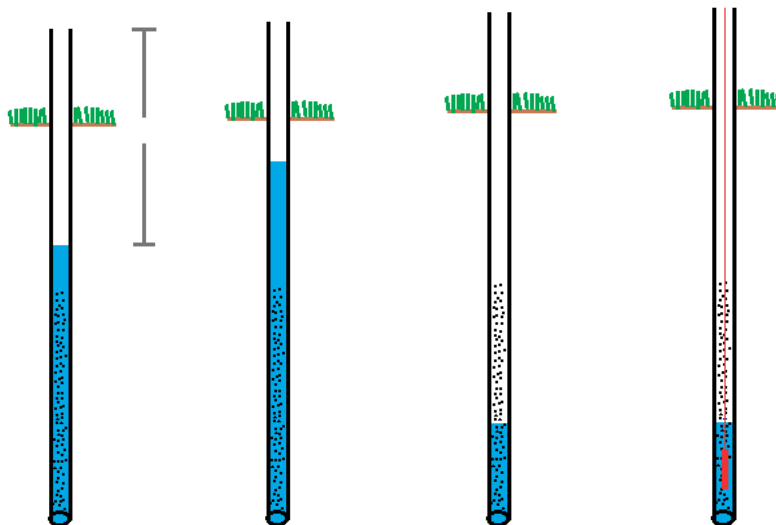
Figure 1a, 1b, 1c, and 1d. The distance between the top of the monitoring tube and the mean groundwater table, the highest water groundwater, the lowest water table, and the correct depth to install above sludge.
